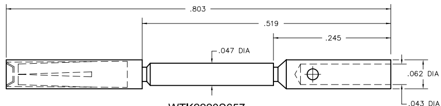
WTK2220S657 SOCKET, CRIMP REMOVABLE, 20 GAGE BARREL
